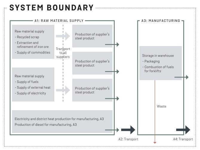
Figure 3. Simplified process tree.
