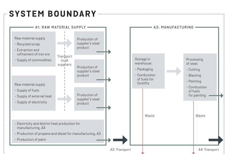
Figure 3. Simplified process tree.
