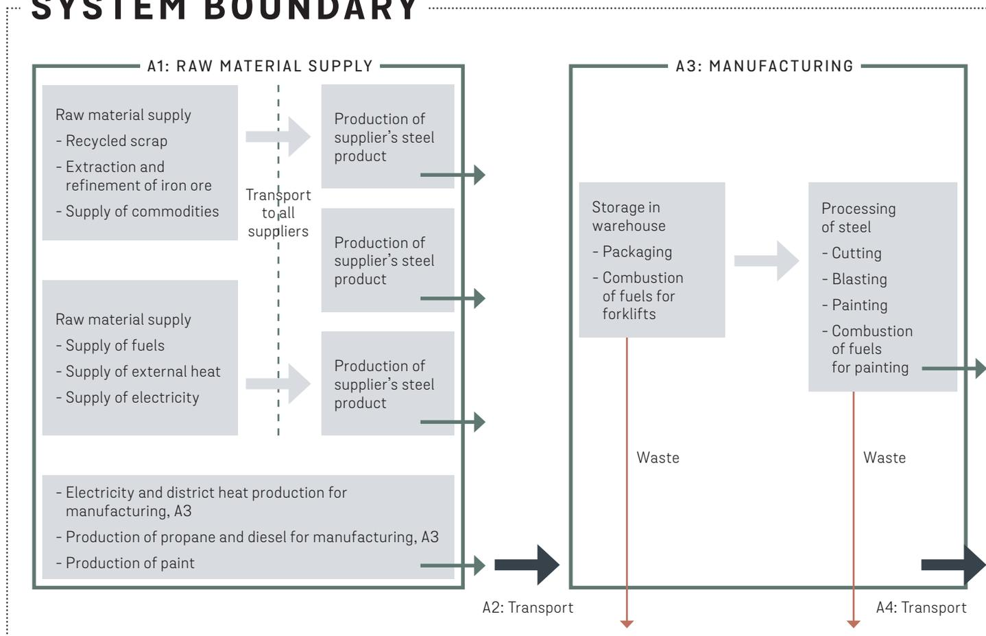
Figure 3. Simplified process tree.
